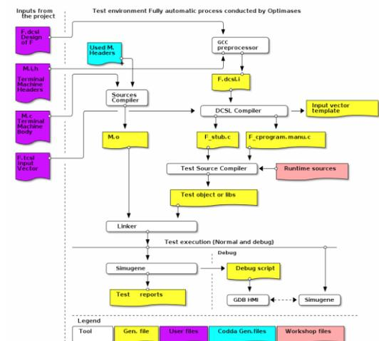
Figure 3: Unit Test automatic process
