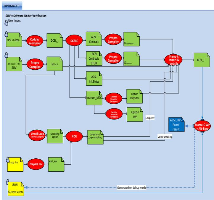
Figure 2: Unit Proof automatic process
